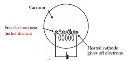
**Heated filament gives out electrons**
